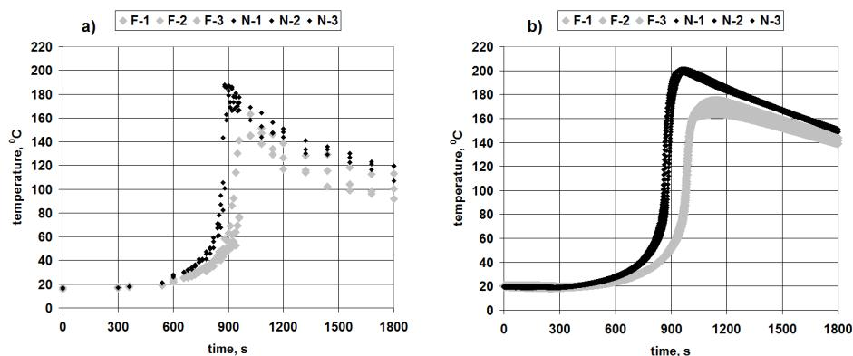
Fig. 3. Temperature-time dependence for curing process of neat polyester resin (des. N) and resin filled with 70 g of fragmented glass fabric (des. F): a) measurement with pyrometer on upper surface of sample, b) measurement with thermocouple in central point inside sample
