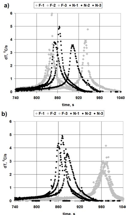
Fig. 4. Temperature-time derivative function dependence versus temperature for curing process of polyester resin: neat (des. N) and filled (des. F), thermocouple measurement: a) 35 g filling, b) 70 g filling
