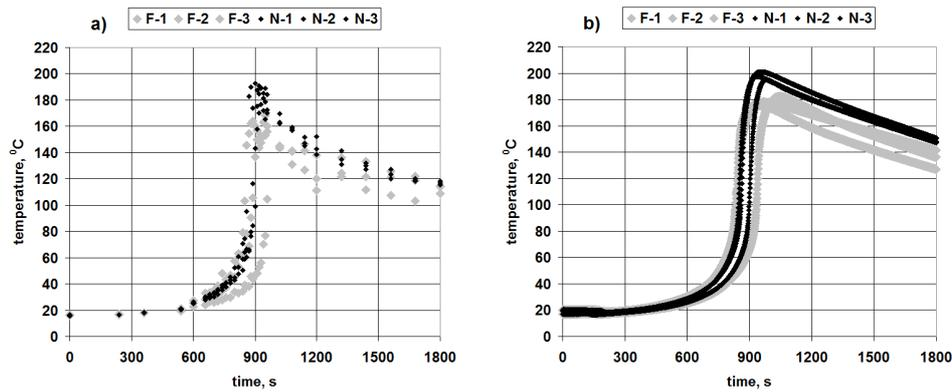
Fig. 2. Temperature-time dependence for curing process of neat polyester resin (des. N) and resin filled with 35 g of fragmented glass fabric (des. F): a) measurement with pyrometer on upper surface of sample, b) measurement with thermocouple in central point inside sample
