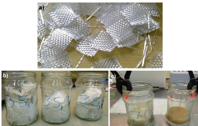
Fig. 1. Realization of resin curing tests: a) pieces of fragmented glass fabric, b) samples of fabric pieces in measuring vessels, c) curing tests - visible sample with pieces of fabric and neat resin sample, thermocouples also visible placed under surface mirror of curing resin
