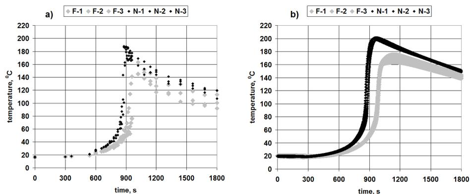
Fig. 3. Temperature-time dependence for curing process of neat polyester resin (des. N) and resin filled with 70 g of fragmented glass fabric (des. F): a) measurement with pyrometer on upper surface of sample, b) measurement with thermocouple in central point inside sample
