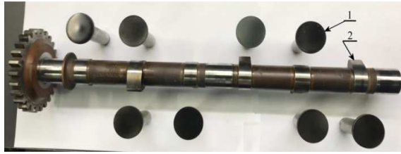
Fig. 7. Camshaft and coated push rods before testing in engine: 1 - push rod, 2 - cam
