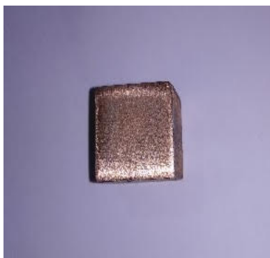
Fig. 2. Copper electrode (ratio: 1:1, size: 18.72 mm x 18.72 mm)
