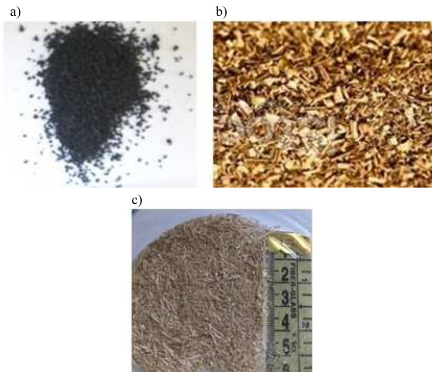
Fig. 1. Macroscopic observations of: a) rubber particles, b) brass particles, c) miscanthus fibers
