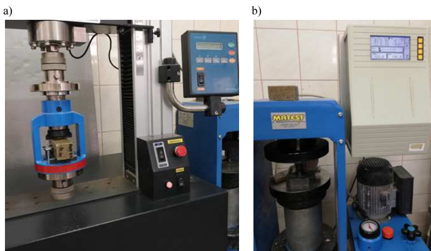
Fig. 3. Machines for testing a) flexural and b) compressive strength
