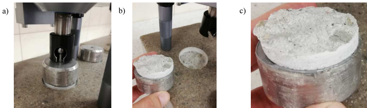
Fig. 8. Adhesion test to concrete: a) sample during test, b) sample after test, c) enlargement – visible cohesive model of detachment in concrete substrate
