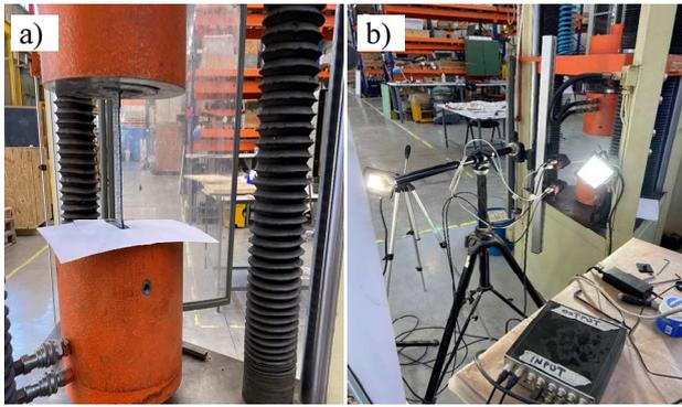
Fig. 3. Galdabini machine used for tensile test (a), digital image correlation instruments (b)
