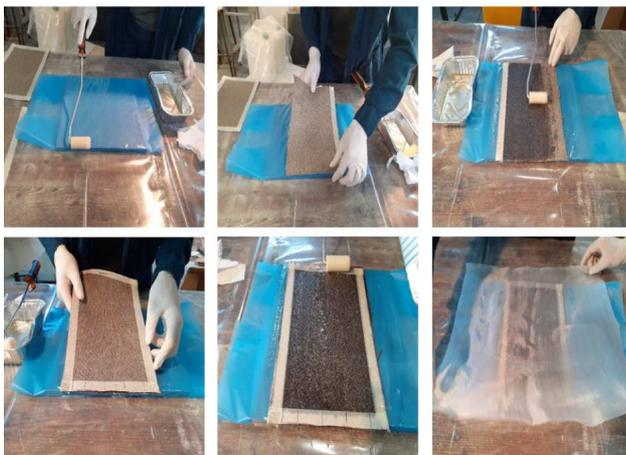
Fig. 2. Sequence of lamination phases
