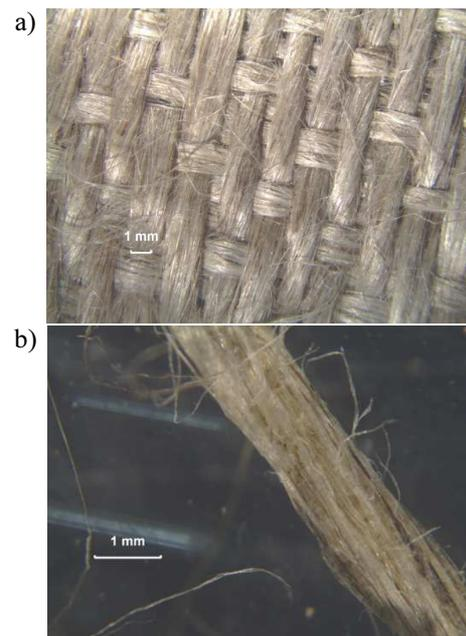
Fig. 1. Micrographs of: a) hemp woven fabric, b) single hemp strand
