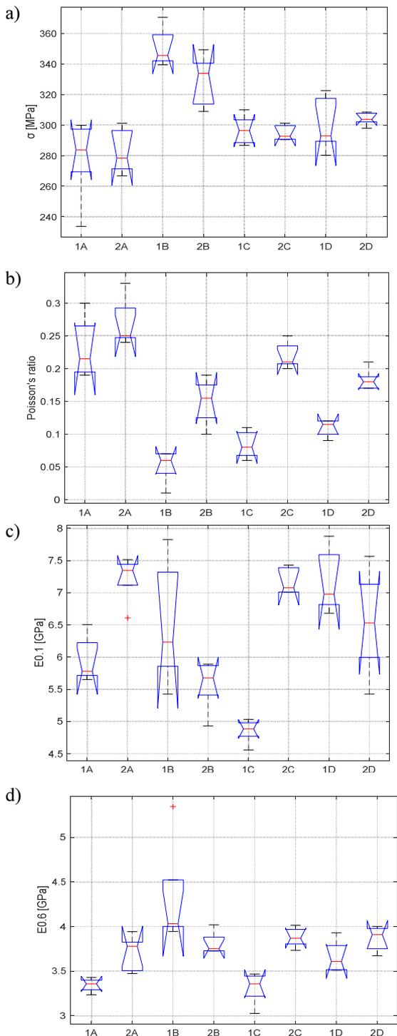
Fig. 9. Box plots of mechanical properties for all tested species: a) tensile strength  $\sigma$ ; b) Poisson's ratio; c) elastic modulus for 0.1 N/N<sub>max</sub>; d) elastic modulus for 0.6 N/N<sub>max</sub>.
