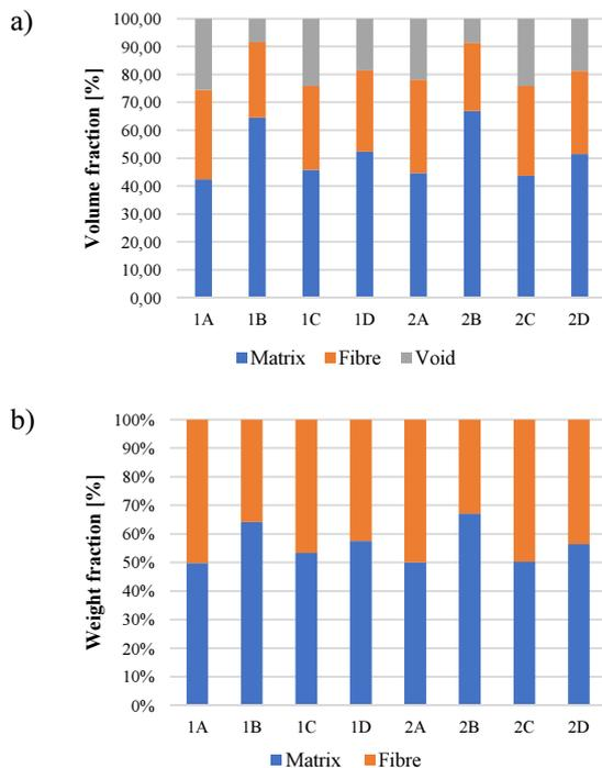
Fig. 4. Histograms of: a) volume percentage of matrix, fibres and voids, b) weight percentage matrix and fibre of all produced composites
