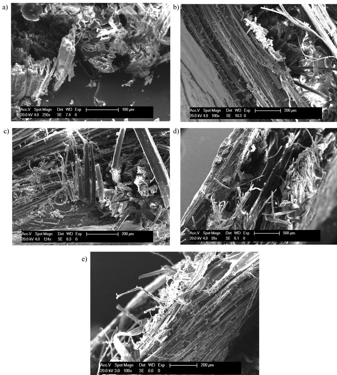
Fig. 6. Images obtained by SEM for fracture surfaces of some of specimens after tension test: a) specimen 1A1; b) specimen 1B2; c) specimen 2B4; d) specimen 1C3; e) specimen 2C5
