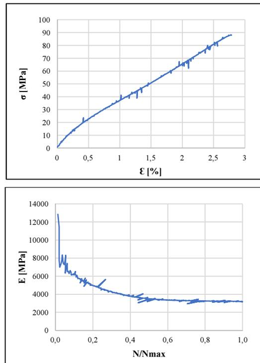
Fig. 5. Stress-strain in longitudinal direction for generic samples 1A1
