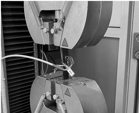
Fig. 6. Unidirectional specimen during tensile test
