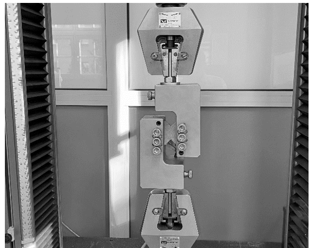
Fig. 8. Specimen during shear test
