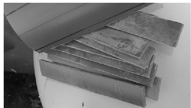
Fig. 4. PVC specimens cut from pipe
