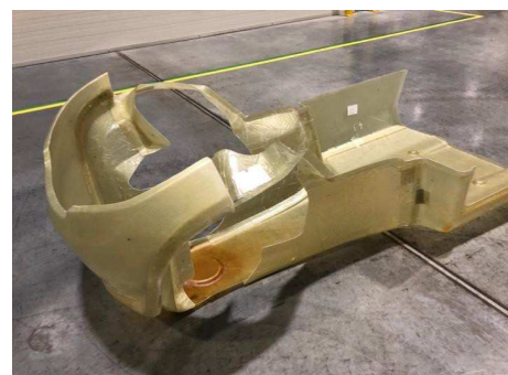
Fig. 12. TRIGGO body parts fabricated as part of the project, connected in layout that matches assumptions
