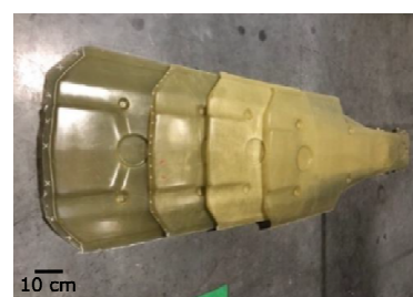
Fig. 9. TRIGGO vehicle parts made in single-sided heated mold in membrane press with membrane vacuum assistance (casing bottom)
