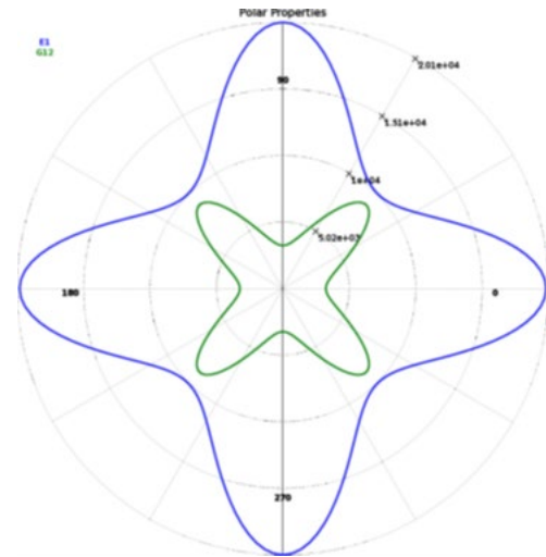
Fig. 1. Young's and Kirchhoff's modules as a function of fibre direction for single layer of glass fabric
