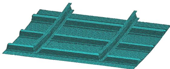
Fig. 1. FEM meshing of the panel
