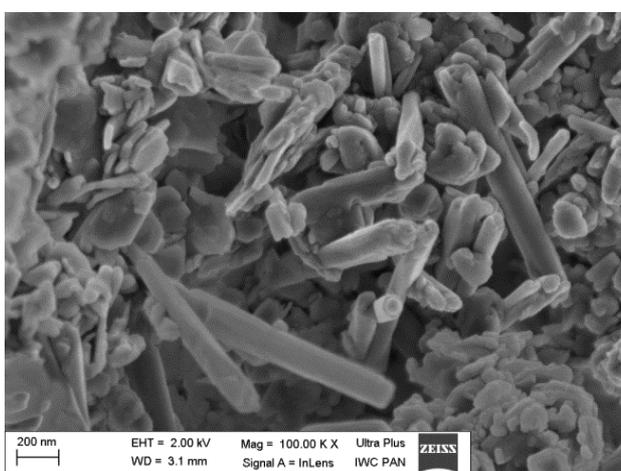
Fig. 2. Halloysite microstructure
