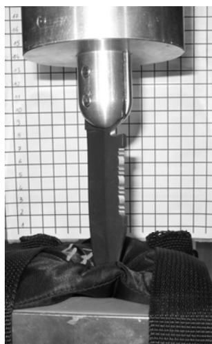
Fig. 3. Blade used in knife penetration resistance test
