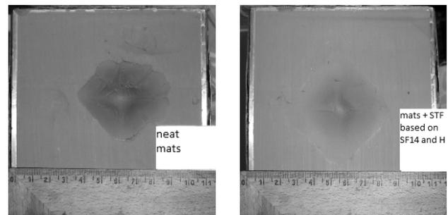
Fig. 8. Photographs of deformations in ballistic plasticine
