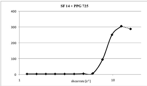
Fig. 5. Viscosity curve of reference sample based on SF14 and PPG 725
