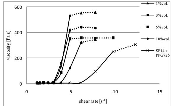
Fig. 7. Viscosity curves of STF based on SF14 doped by modified halloysite dispersed in PPG 725
