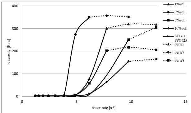
Fig. 6. Viscosity curves of STF based on SF14 doped halloysite dispersed in PPG 725
