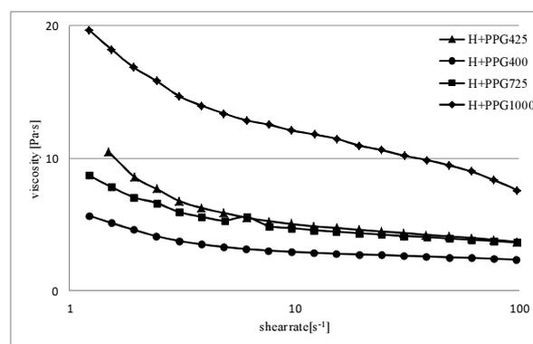
Fig. 4. Viscosity curves of STF based on halloysite and PPG
