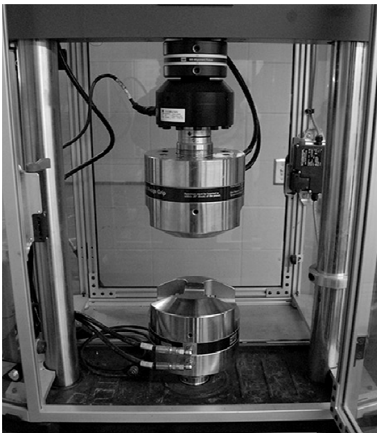
Fig. 6. Experimental testing stand for composite structures with delamination
