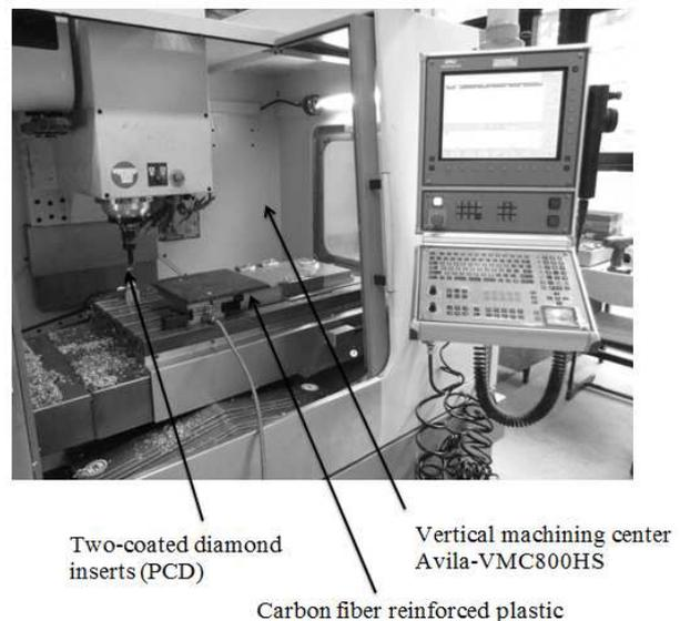
Fig. 1. Scheme of test stand
