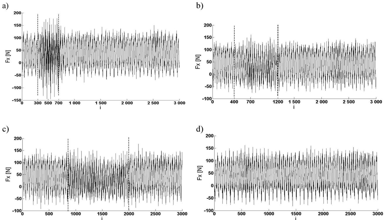
Fig. 3. Cutting forces  $F_x$  obtained by milling flat surface: a) with hole diameter  $\phi 2$  mm, b) with hole diameter  $\phi 4$  mm, c) with hole diameter  $\phi 6$  mm, d) without hole
