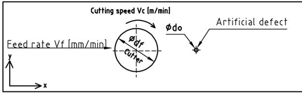
Fig. 2. Scheme of milling process with artificial defect (hole)  $\phi d_o$
