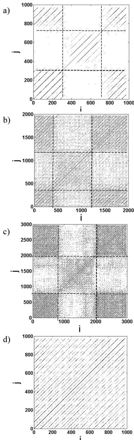
Fig. 4. Recurrence plots obtained from cutting force signals: a) with hole diameter  $\phi$  2 mm ( $m = 5, d = 8, \varepsilon = 20$ ), b) with hole diameter  $\phi$  4 mm ( $m = 4, d = 9, \varepsilon = 20$ ), c) with hole diameter  $\phi$  6 mm ( $m = 4, d = 9, \varepsilon = 20$ ), d) without hole ( $m = 4, d = 8, \varepsilon = 20$ )
