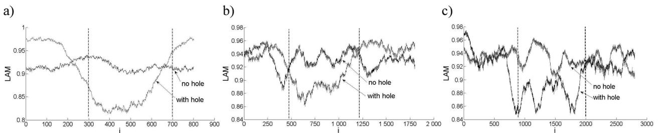
Fig. 7. Laminarity LAM of recurrence plot: a) with hole diameter  $\phi$  2 mm ( $m = 5, d = 8, \varepsilon = 20$ ) and without hole ( $m = 4, d = 8, \varepsilon = 20$ ), b) with hole diameter  $\phi$  4 mm ( $m = 4, d = 9, \varepsilon = 20$ ) and without hole ( $m = 4, d = 9, \varepsilon = 20$ ), c) with hole diameter  $\phi$  6 mm ( $m = 4, d = 9, \varepsilon = 20$ ) and without hole ( $m = 4, d = 9, \varepsilon = 20$ )
