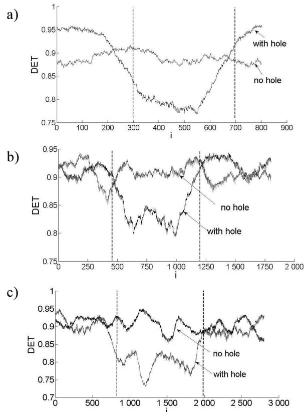
Fig. 5. Determinism *DET* of recurrence plot obtained by milling a flat surface: a) with hole diameter  $\phi$  2 mm ( $m = 5, d = 8, \varepsilon = 20$ ) and without hole ( $m = 4, d = 8, \varepsilon = 20$ ), b) with hole diameter  $\phi$  4 mm ( $m = 4, d = 9, \varepsilon = 20$ ) and without hole ( $m = 4, d = 9, \varepsilon = 20$ ), c) with hole diameter  $\phi$  6 mm ( $m = 4, d = 9, \varepsilon = 20$ ) and without hole ( $m = 4, d = 9, \varepsilon = 20$ )
