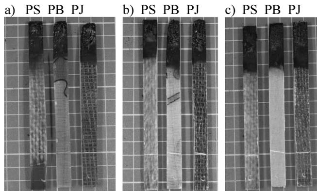
Fig. 5. View of samples after burning: a) 3 layers of reinforcement, b) 6 layers of reinforcement, c) 9 layers of reinforcement
