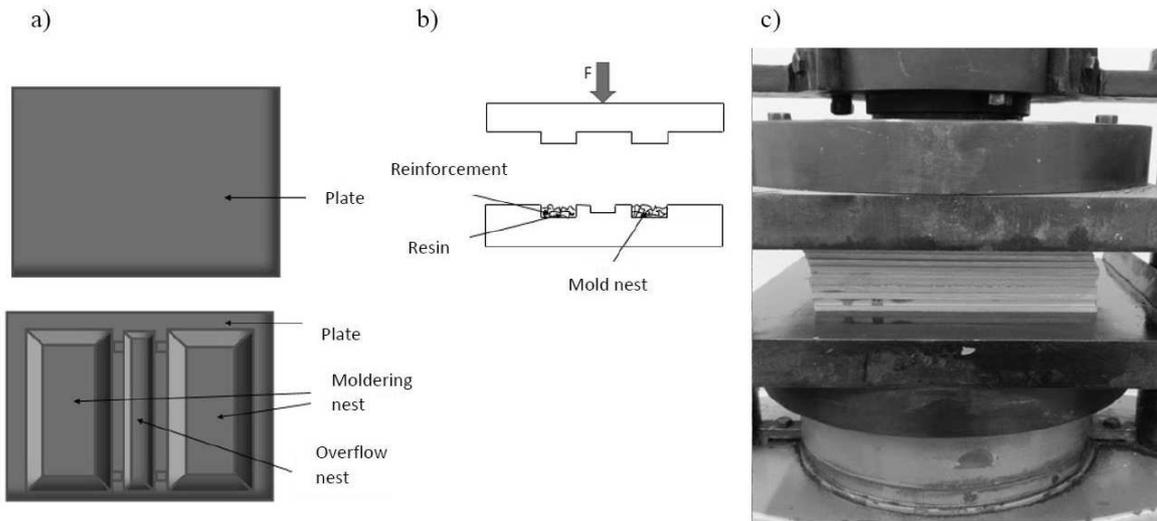
Fig. 3. Project of mould (a), sectional view (b), view of mould mounted on pressing station (c)
