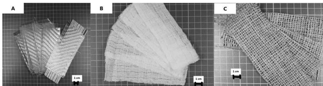
Fig. 2. Materials used for reinforcement: A) glass tissue (PS), B) cotton (PB), C) jute (PJ)
