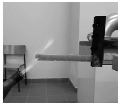
Fig. 4. Burning test in compliance with UL 94 HB
