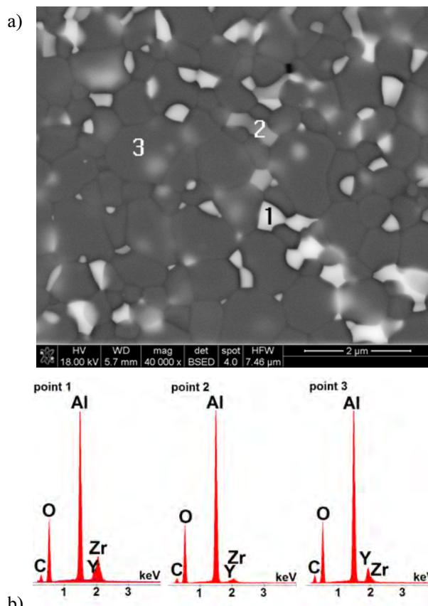
Fig. 2. Typical SEM image of AYZ5 composite (a); EDS spectra indicates chemical composition qualitatively in marked places (b)
