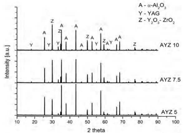
Fig. 1. XRD diffractograms of obtained composite sinters
