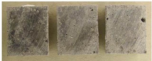
Fig. 4. Macrostructure of longitudinal section of Mg3Al-GCp composite samples remelted at temperature of 610°C during 30, 60, and 90 minutes
