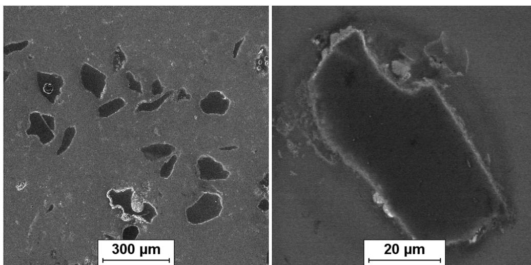
Fig. 2. Micrographs of stir cast Mg<sub>2</sub>ZnZrRE-GCp composite, SEM
