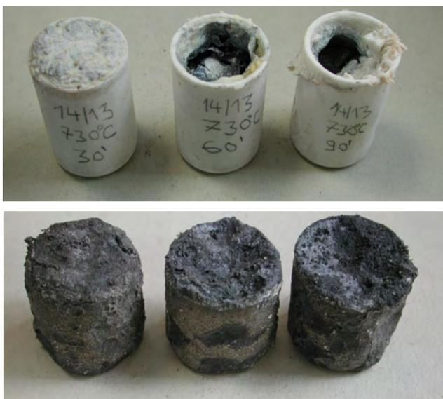
Fig. 3. View of composite samples after remelting and cooling: a) in ceramic crucibles, b) after crucible removal
