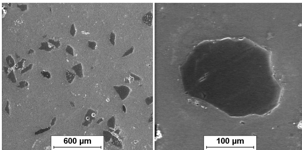
Fig. 1. Micrographs of stir cast Mg<sub>3</sub>Al-GCp composite, SEM
