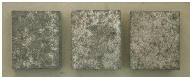
Fig. 9. Macrostructure of longitudinal section of Mg<sub>2</sub>ZnZrRE-GCp composite sample remelted at temperature of 640°C during 30, 60 and 90 minutes
