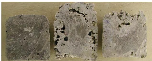
Fig. 7. Macrostructure of longitudinal section of Mg<sub>3</sub>Al-GCp composite samples remelted at temperature of 730°C during 30, 60, and 90 minutes
