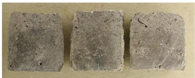
Fig. 6. Macrostructure of longitudinal section of Mg3Al-GCp composite samples remelted at temperature of 690°C during 30, 60, and 90 minutes
