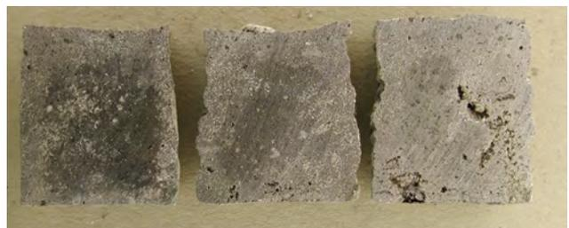
Fig. 5. Macrostructure of longitudinal section of Mg3Al-GCp composite samples remelted at temperature of 640°C during 30, 60, and 90 minutes
