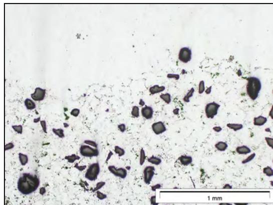
Fig. 12. Micrograph of Mg<sub>2</sub>ZnZrRE-GCp composite sample remelted at 690°C for 30 minutes, metal zone without particles (top) and zone with particles segregated at bottom of crucible (bottom), LM
