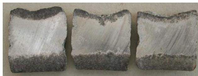
Fig. 11. Macrostructure of longitudinal section of Mg<sub>2</sub>ZnZrRE-GCp composite sample remelted at temperature of 730°C during 30, 60, and 90 minutes
