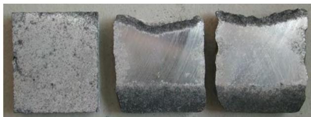
Fig. 10. Macrostructure of longitudinal section of Mg<sub>2</sub>ZnZrRE-GCp composite sample remelted at temperature of 690°C during 30, 60, and 90 minutes
