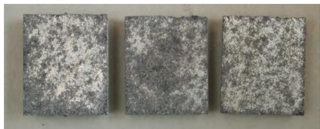
Fig. 8. Macrostructure of longitudinal section of Mg<sub>2</sub>ZnZrRE-GCp composite sample remelted at temperature of 610°C during 30, 60 and 90 minutes
