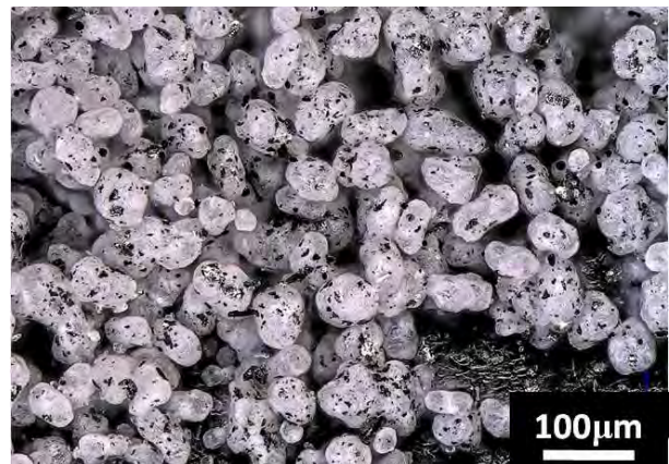
Fig. 4. Image of PA-G composite powder particles after 8 - hour mixing time
