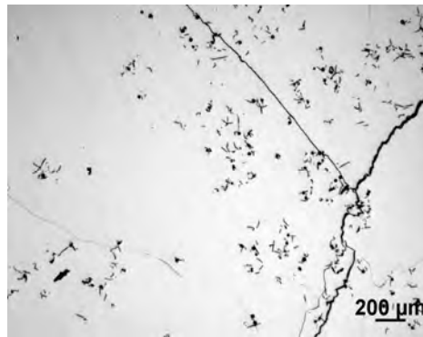
Fig. 4. Microscopic image of Ni_3Al/C composite sample surface with precipitates of nodular graphite eutectic revealed by etching in "aqua regia". Sample cast in metal mould, very rapid cooling in liquid nitrogen at rate of about 100 K/s
