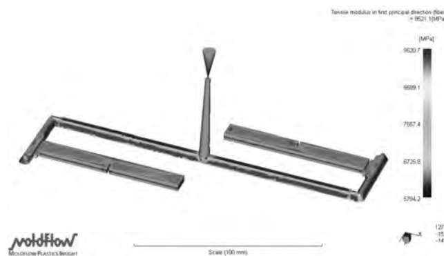
Fig. 5. Changes in Young modulus for part from composite of PA6 with 25% glass fibre content
