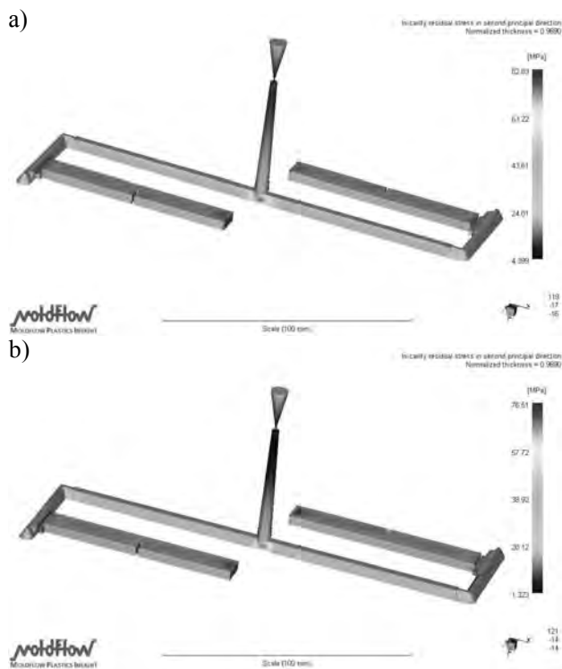
Fig. 3. Residual stress distribution for PA6 with 25% glass fibre content: a) for holding pressure of 30 MPa, b) for holding pressure of 50 MPa
