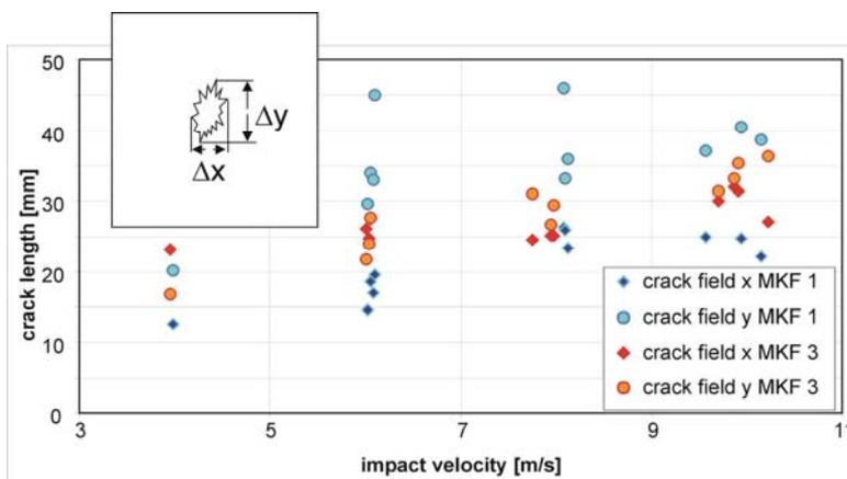
Fig. 8. Fracture extents of different MKF dependent on the impact velocity
