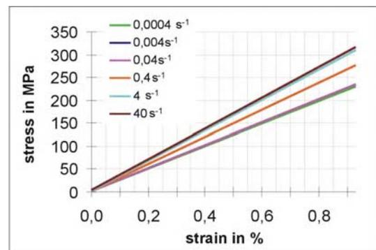
Fig. 5. Strain rate dependent stress-strain diagrams of glass fibre reinforced specimen (linearised)
