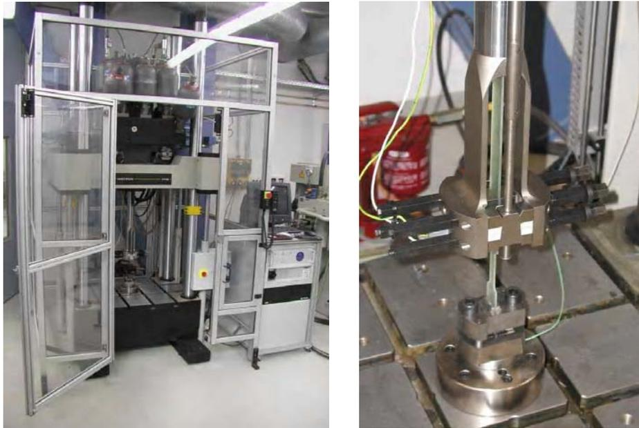
Fig. 1. Servo-hydraulic high-speed test unit at ILK
