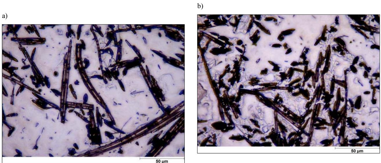
Fig. 5. Microstructure of AE42+Saffil in fibre plane: a) as squeeze cast, b) after creep
