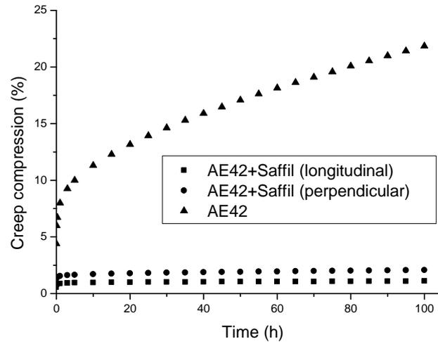
Fig. 2. Creep curves of squeeze cast specimens at 200°C and 100 MPa load
