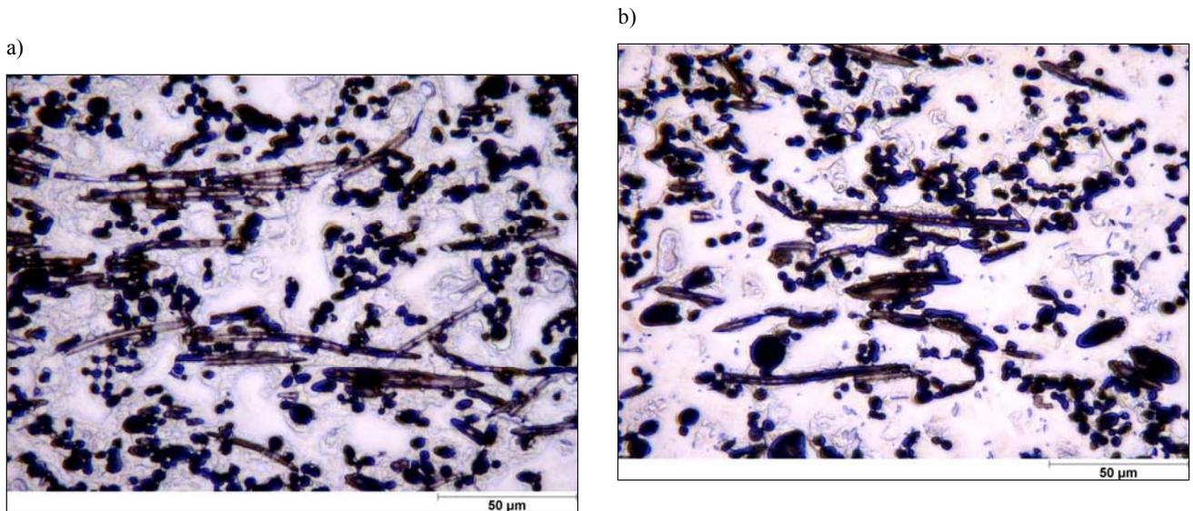
Fig. 4. Microstructure of AE42+Saffil perpendicular to fibre plane: a) as squeeze cast, b) after creep
