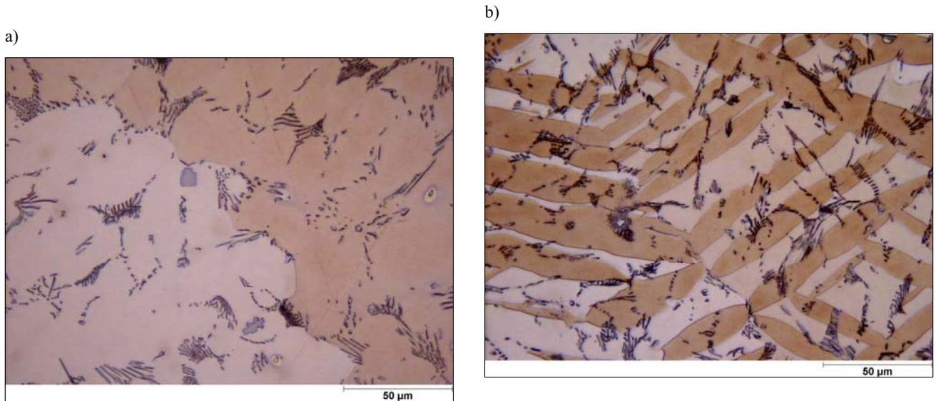
Fig. 3. Microstructure of AE42: a) as squeeze cast, b) after creep
