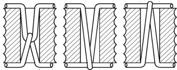
Fig. 3. Variation of the yarn tension with the double locked stitch technology [2]
