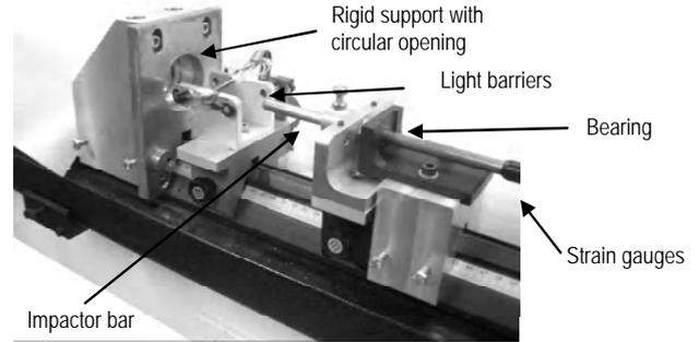
Fig. 1. Impact-bending-test device (IBT) with rigid support [3] (without specimen)
