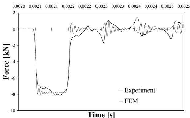
Fig. 2. Comparison between experimental and FEA results of the impact: projectile - impactor bar
