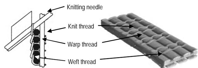
Fig. 5. MKF type 1, left: basic architecture (schematic) [6], right: CT-scan [3]
