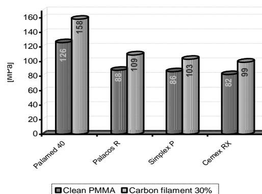
Fig. 5. Compressive strength  $R_c$  [MPa] for bone cements and well as cements with carbon fibre
