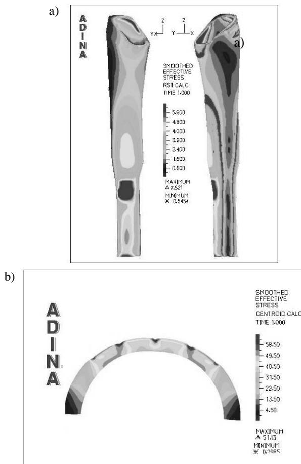
Fig. 3. Map of reduced stress  $\sigma$  [MPa] for polymethyl methacrylate
