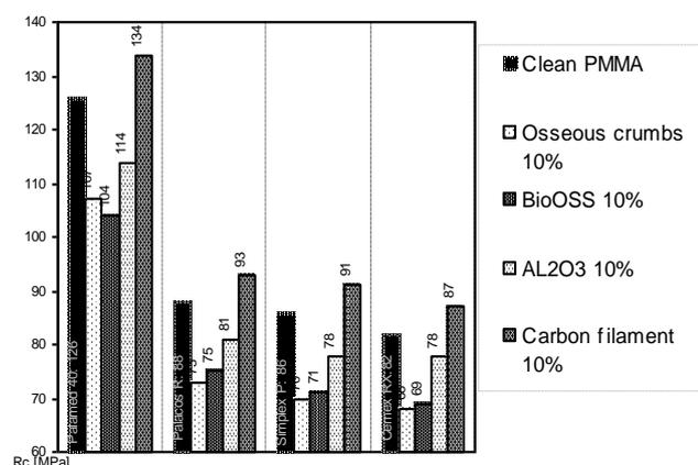
Fig. 4. Compressive strength  $R_c$  [MPa] for bone cements with different fillers
