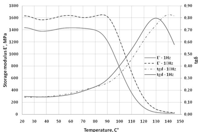
Fig. 7. DMTA thermogram for the material with the highest storage modulus  $E'$  and the mechanical loss factor
