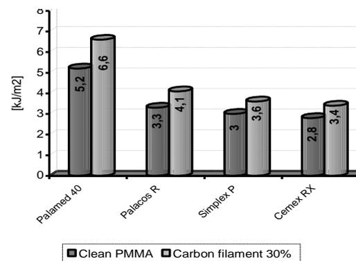
Fig. 6. Impact strength in PMMA/carbon fibre composite
