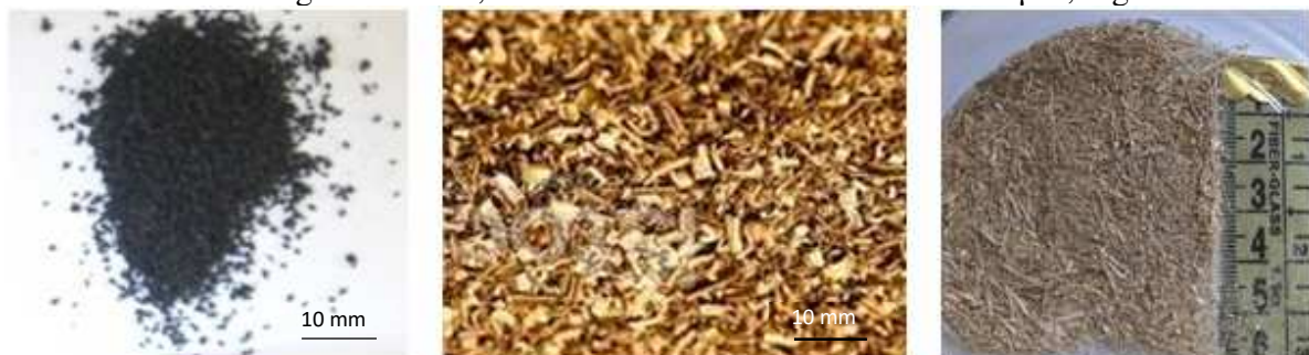
Figure 1. Macroscopic observations of: a) rubber particles, b) brass particles, c) miscanthus fibers
