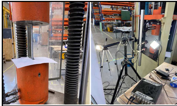
Fig. 3. Left, Galdabini machine used for tensile test, right, digital image correlation instruments.
