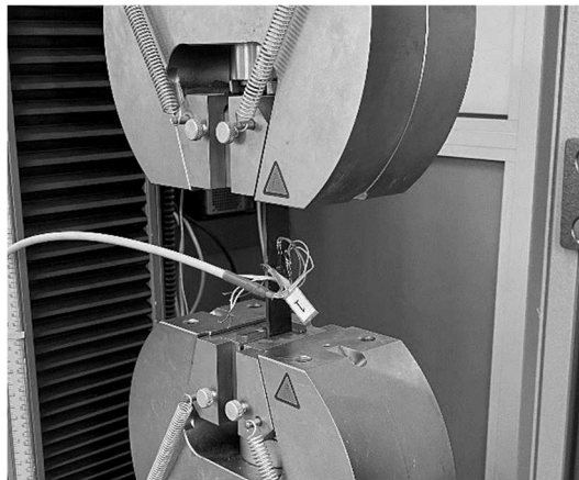
Fig. 6 Unidirectional specimen during tensile test
