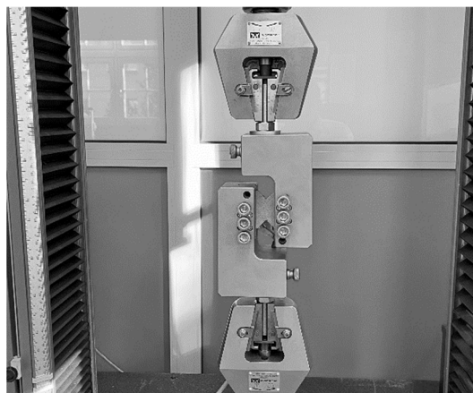
Fig. 8. Specimen during shear test
