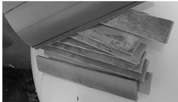
Fig. 4. PVC specimens cut from pipe
