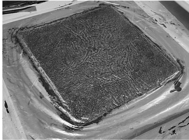
Fig. 3. Plate made out of glass fiber mat and polyester resin after hand layup
